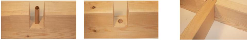
robots. You can purchase one from <http://botbrain.com> (shameless plug!). The BotBrain Maze uses 2x4 lumber that is held together with pegs and holes. It slides together and comes apart easily and is heavy enough to be used without taping down.
