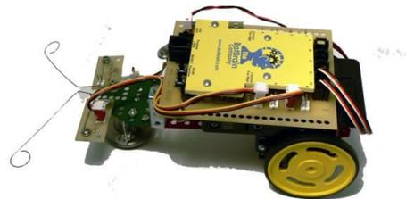
**Programming Dumb Luck** This program uses two test condition tiles, one for each sensor. This particular program assumes that the right sensor is in 2, and the left is in pin 1. The logic here is to check the pin one sensor, if it hit something, back up and turn right. If not, check the pin 2 sensor. If it hit something, backup and turn left. If not, drive forward. The trick here is to adjust the time of the turns until the robot makes it through the maze
